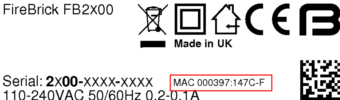
Figure B.1. Product label showing MAC address range
