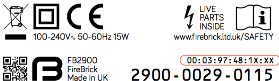
Figure C.1. Product label showing MAC address range
