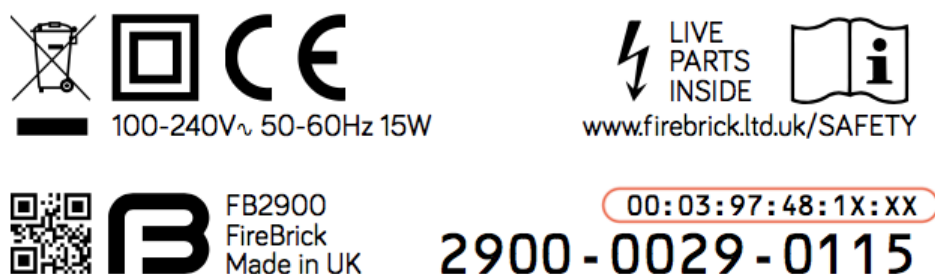
Figure C.1. Product label showing MAC address range
