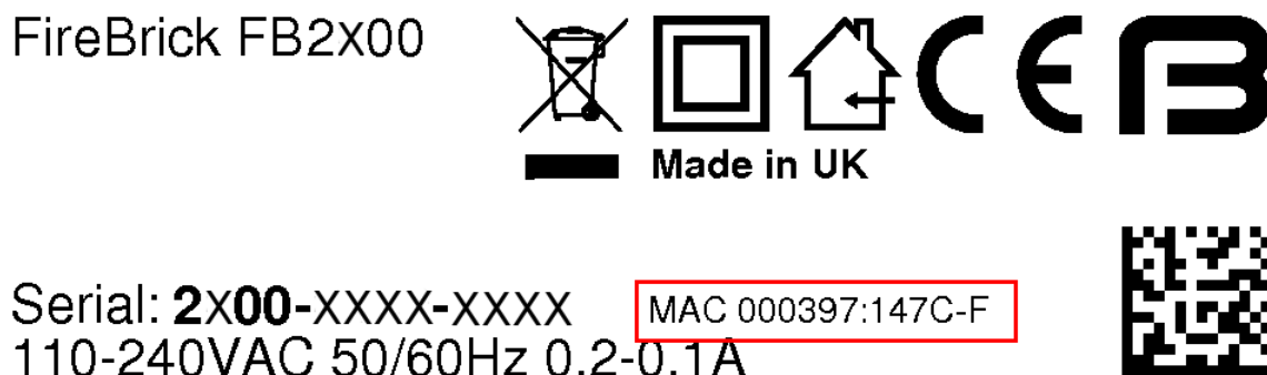
Figure C.1. Product label showing MAC address range
