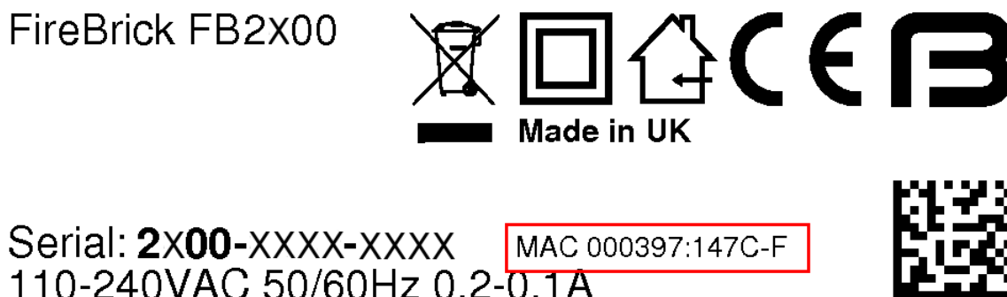
Figure C.1. Product label showing MAC address range
